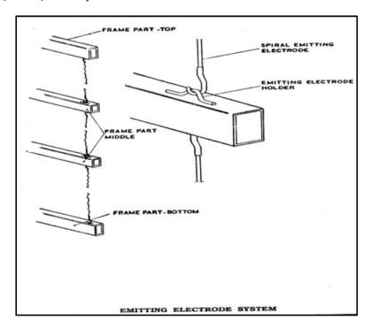
Contractor shall erect, position, perform alignment and welding/bolting/fixing/clamping of the emitting electrode frame work system as shown in figures above with standard erection procedure and gap/distance or other quality parameter or critical dimension considering operation and or erection of ESP will be maintaining as per standard practice.
