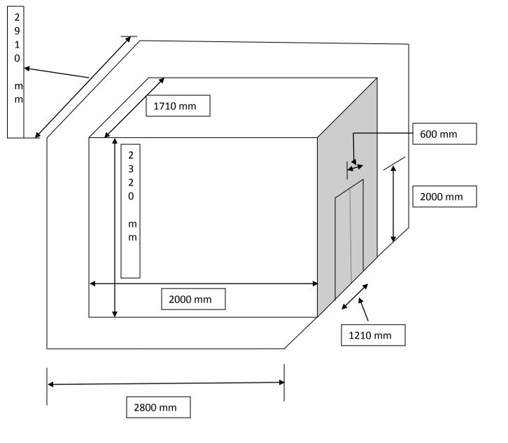
UNIT -1 BOILER LIFT CAR DIMENSIONS
